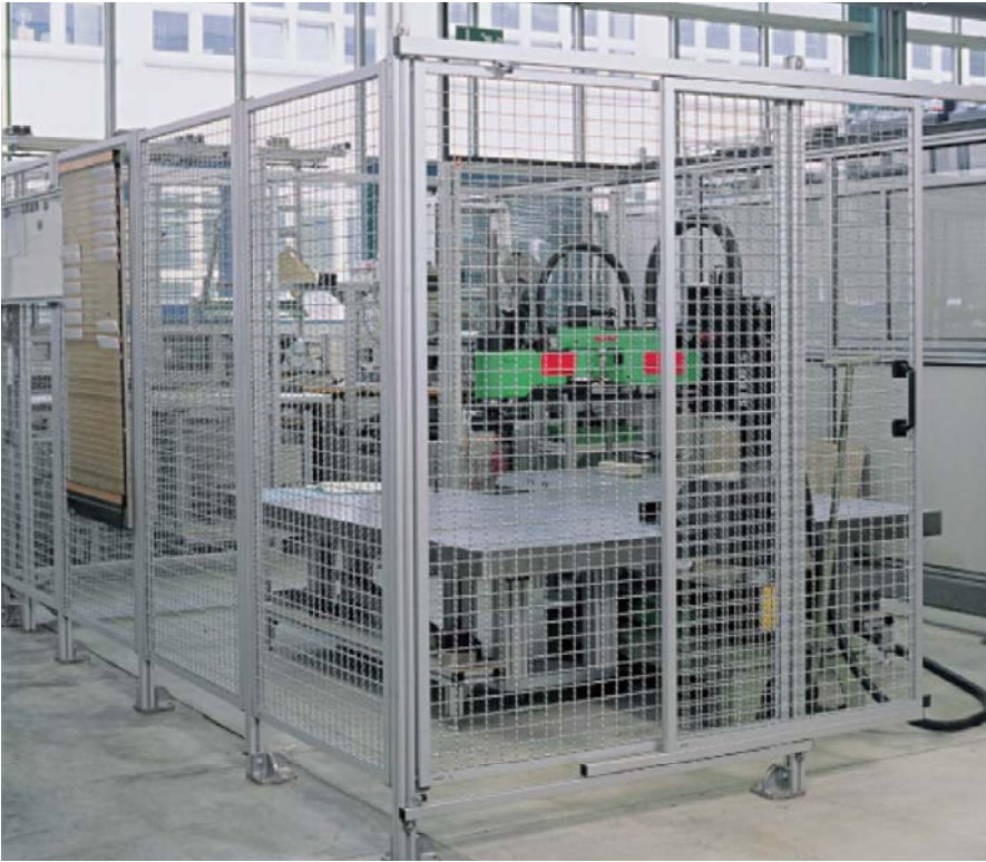
Protective barriers for machine 机器设备外围防护
